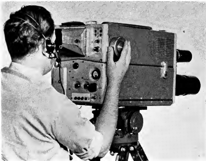
Fig. 3. Television cameral head, showing major controls.
